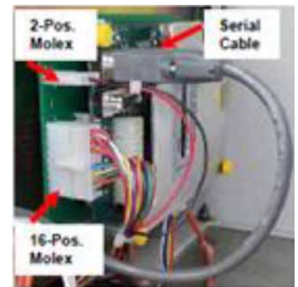
STEP 9. Plug the connectors back in.
