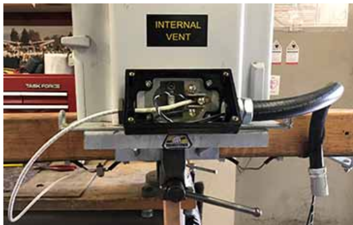
Figure AP 510–9: CPT Grounding Details for Option 2
