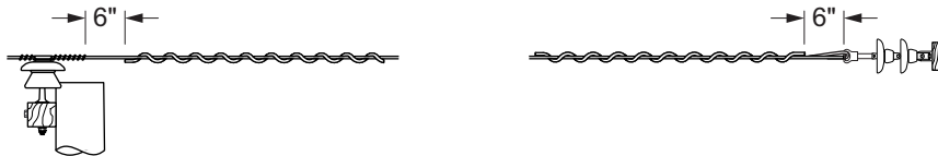
Figure 460-2.1: Two Vibration Dampers Per Conductor — Span Length 300'–800'
