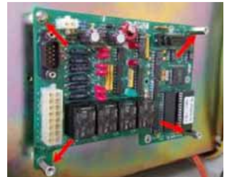
STEP 3. Remove (3) standoffs and screw.
