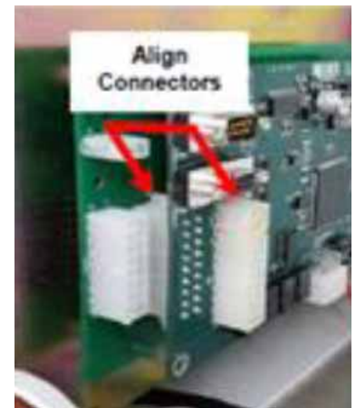
STEP 6. Mount new RTU3211.
