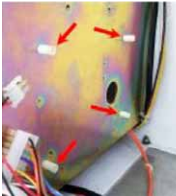
STEP 4. Leave (4) plastic standoffs on side wall.
