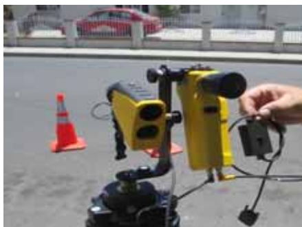
Figure 6.2: Remote Trigger with TruPulse 360
