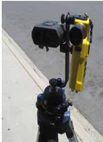
Figure 8: Bracket Attached to Tru Pulse 360R and RD 1000
